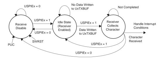
Figure 14–7. SPI Slave Receive-Enable State Diagram
